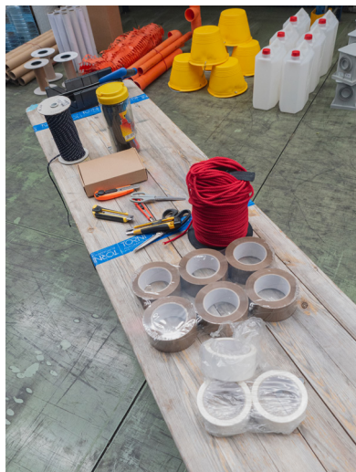
Fig.66 To make the assembly and construction of the typologies easier, each group was provided with materials that did not require special technical skills to use. This approach was influenced by typical protest construction practices, where quick and accessible methods are adopted to ensure inclusive participation. Materials such as tape, ropes, straps and zip ties were suggested to allow for quick and adaptable assemblies, responding to immediate needs and offering practical and replicable solutions.
